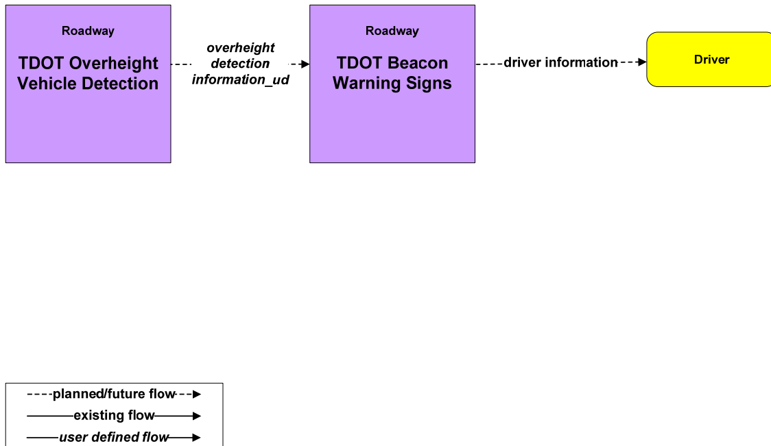
Figure B2 – ATMS01 – Network Surveillance: TDOT Overheight Vehicle Detection
